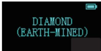
Type IIa, HPHT / CVD - IaB, IIa, IIb, the diamond may be synthetic or color enhanced by HPHT treatment. Recommend to send the stone to a gem laboratory for further examination (Fig. 21).
