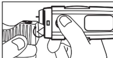
Be sure that the stone is well mounted and it is in contact with its metal setting or mounting. A stone that is very loose may result in inaccurate reading.
