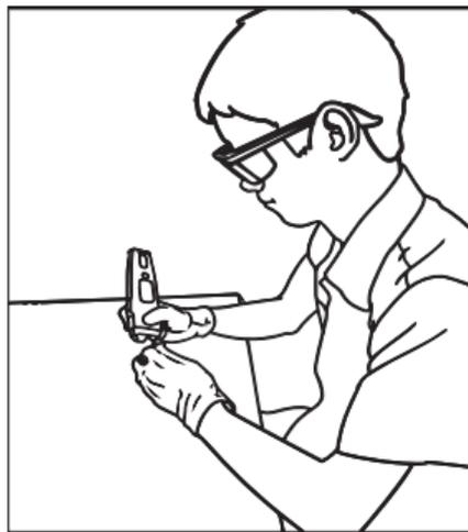
d. Remove the protective cap (1) from the probe tip prior to performing the test as shown in (Fig. 4).
