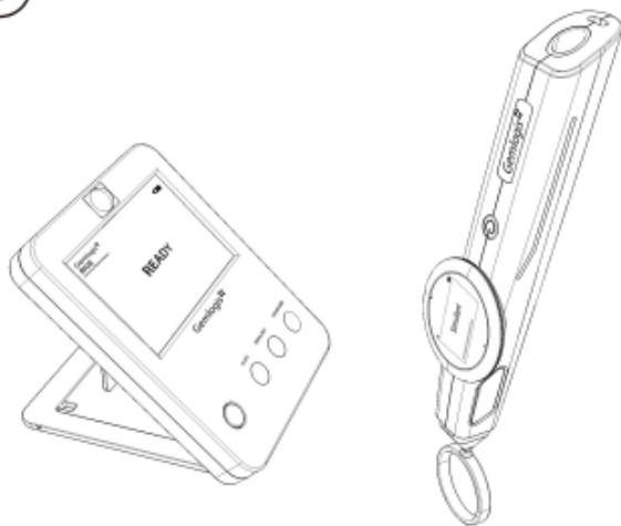
Perform test on mounted stone . Make sure there is a clear path between IR transmitter and receiver
