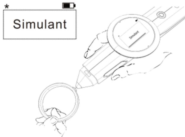
Perform test on mounted stone, hold the jewelry with one hand and the tester with other hand.
