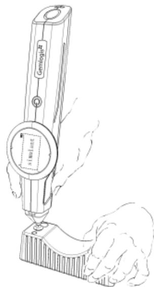
To test loose gemstone , place the gemstone on the metal stone rest and hold it with one hand while holding the tester with the other hand.
